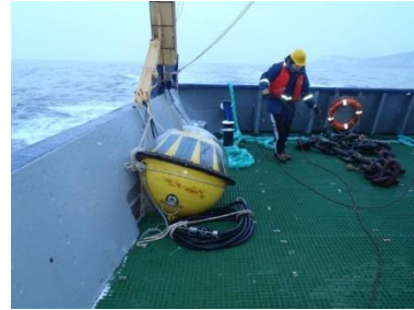
Figure 3: TRIAXYS Directional Wave Buoy used to measure the wave height.
